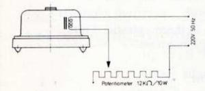
Fig. 4 Adjustment of output with potentiometer.
