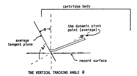
Use the VTA dial (set the lever at 0 degrees) and set the height of the tonearm such that the tonearm wand is parallel to the surface of a record. Then adjust the VTA dial to -1 degrees. This will match the cartridge's vertical angle with that of the record.
