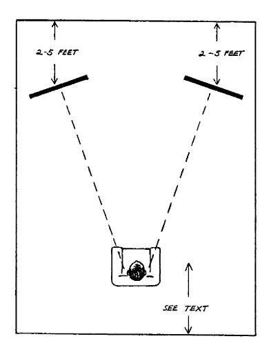
Slight midrange frequency balance changes can be obtained by pointing the speakers slightly away from the listening position. This balance can also
