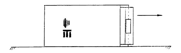
After removing the speaker from its carton it can be leaned against a wall standing up or placed with the front face of the speaker lying flat on carpet. then the black strapping should be removed. These straps tie the feet (wrapped in paper) the baffles (black triangular boards) and the grill cloth (covered by a large cardboard sheet) to the speaker. After the strapping is removed these will seperate from the speaker.
