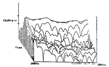
Vertical: 12dB/div with base of display at 13.6dB 0dB is located at .00002 pascals
