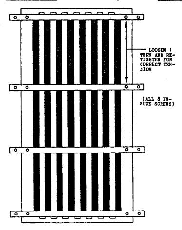
The idea is not to tighten these screws as much as possible, but rather to temporarily "relax" the entire frame so the Mylar diaphram can recover its original tension.
