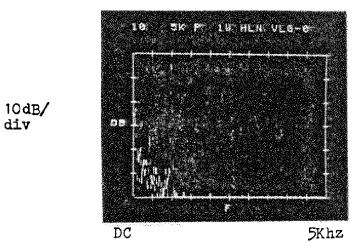
Distortion test-1Khz @ 90dB sine wave Absence of harmonics above 1Khz indicates distortion below .1%. (noise floor of room) Typically measures .03%.
